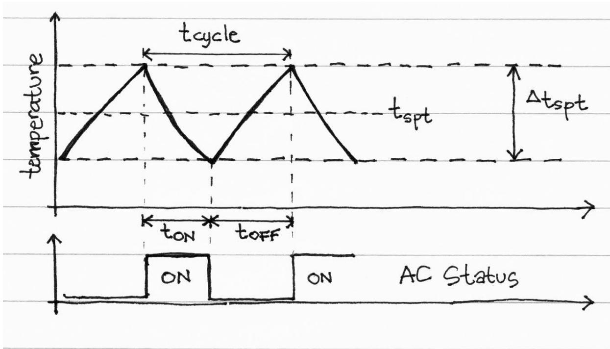
**Figure 4** Indoor air temperature and AC status
