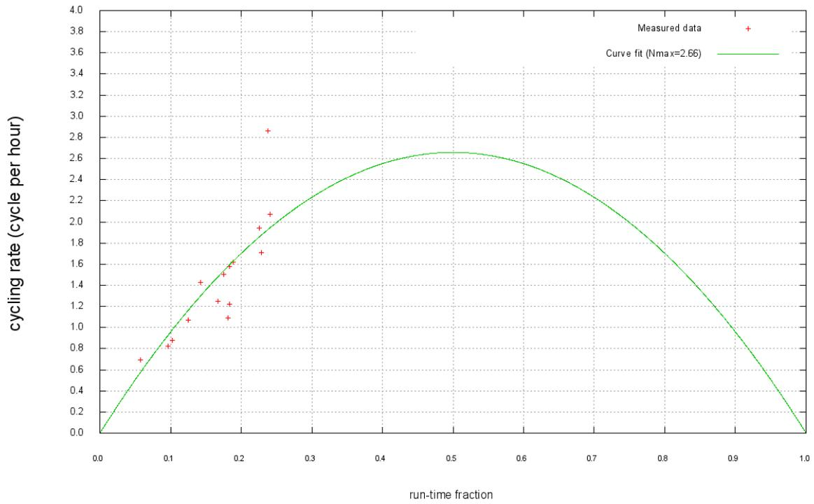
**Figure 5** Calculation of  $N_{max}$  from measurement data.
