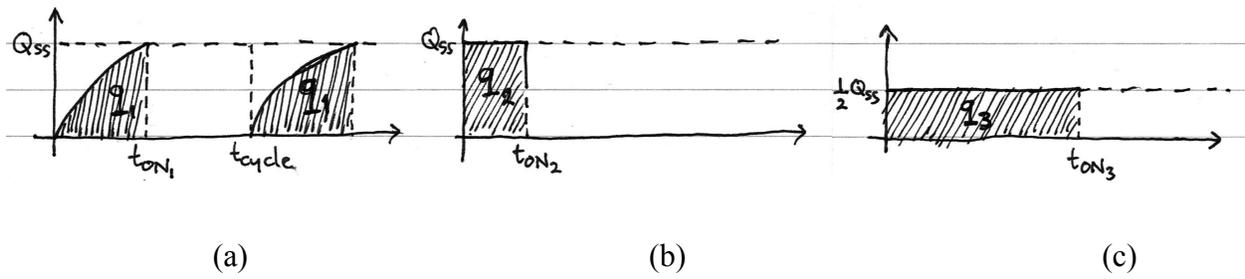
**Figure 3** Quantifying oversizing energy penalty (a) actual cycling case (b) idealized steady-state case with oversized unit (c) idealized steady-state with rightsized unit
